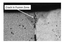
In both types of Nickel plating processes, the plating vendor may decide to add some pixie dust and try to impress you with making a bright Ni plating. The pixie dust is typically proprietary chemicals that turn a dull matt finish on the Ni plating into a bright shiny surface. Unfortunately, the brighteners added are almost always detrimental to the welding process. This is one situation where the welding engineer would be smart and choose to be dull.
