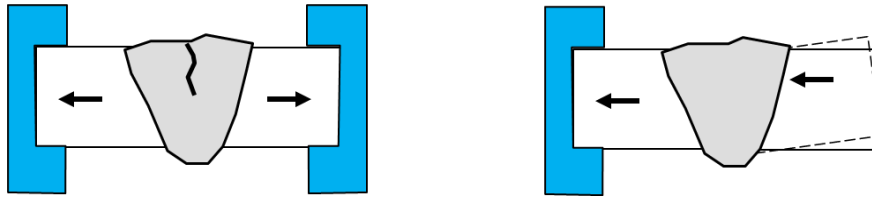
Figure 2. Schematic on left shows two parts being welded with heavy restraint resulting in residual stress in the weld which can lead to cracking. Schematic on the right shows a weld with some degree of freedom to move and relieve contraction stresses.
