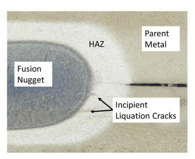
Photo above shows a weld section of a resistance weld in an Inconel alloy. Fusion nugget, HAZ, and parent metal are evident. Also shown are phase separation regions that indicate locations of potential liquation cracks under suitable stress conditions.
