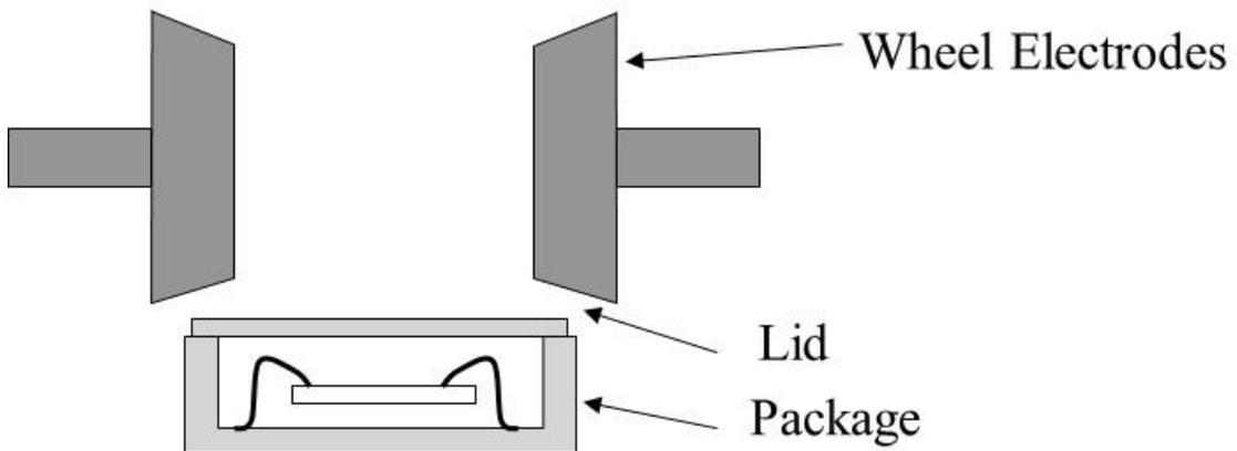
Figure 2. Schematic showing roll-spot welding used for sealing lids. The round wheel electrodes traverse along the length of the package making overlapping spots.
