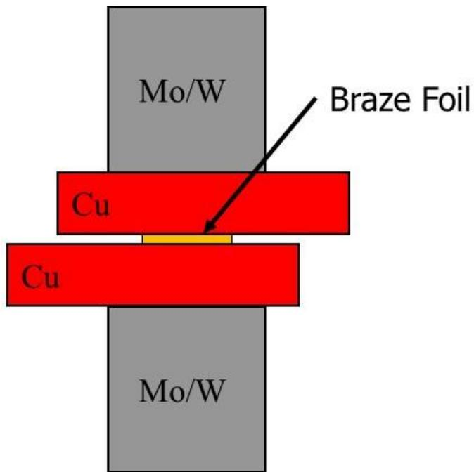
Figure 1. Schematic showing two copper pieces sandwiching a Sil-Phos foil and being resistance brazed by two molybdenum or tungsten electrodes.
