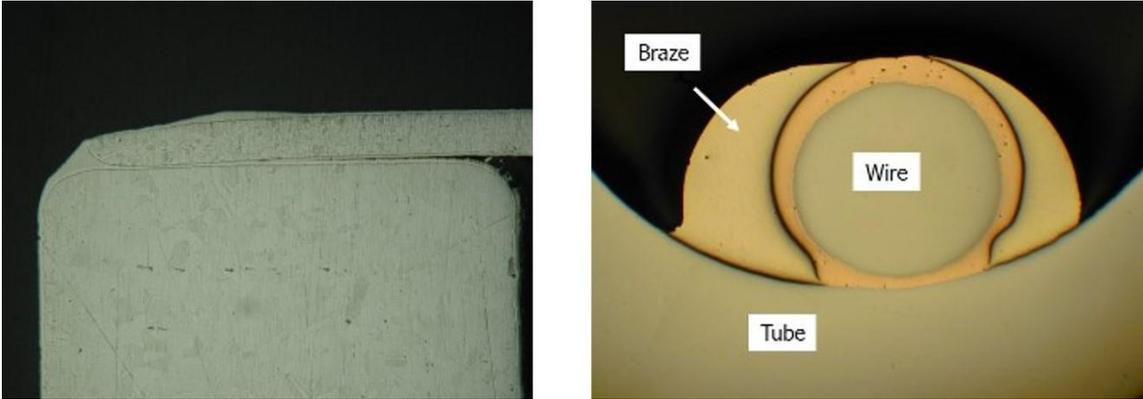
Figure 3. Section of braze joint on the left show a braze between kovar lid and base. Flow of Ni and Au plating to form a fillet is evident. Section on the right shows a braze joint that is actually a solid-state bond on the inside, even though a braze fillet is visible on the outside.
