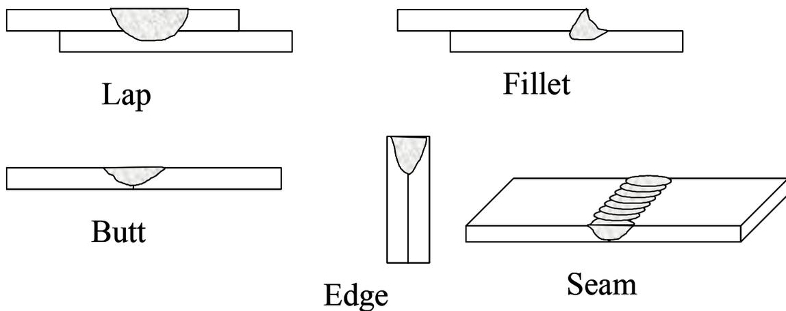
Figure 4. Schematics of weld configurations for laser welding. Fusion zones are shaded. Any of the configurations can be seam welded with overlapping spot welds.
