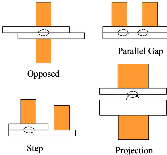
Figure 2. Weld configurations commonly used for resistance welding. Electrodes are shown red in color and the weld location is shown as an ellipse with a dashed line boundary.
