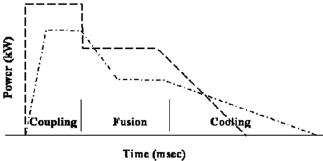
Figure 1. Anatomy of a laser pulse showing coupling, fusion, and cooling segments for two typical pulse shapes. Pulse times, shapes, and energy/power per segment, can vary based on application.
