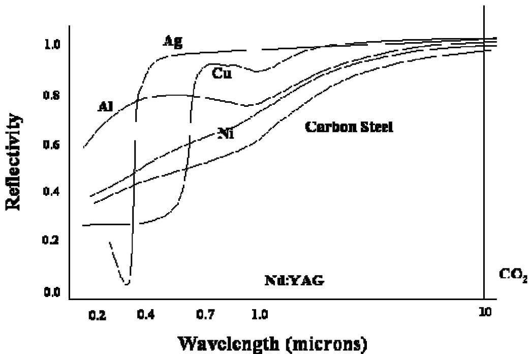
Figure 2. Absorption of laser energy by metals at room temperature. Note that metals that are white in color such as silver are good reflectors of YAG laser light. Metals that are grey in color such as steels are good absorbers of laser light at room temperature.
