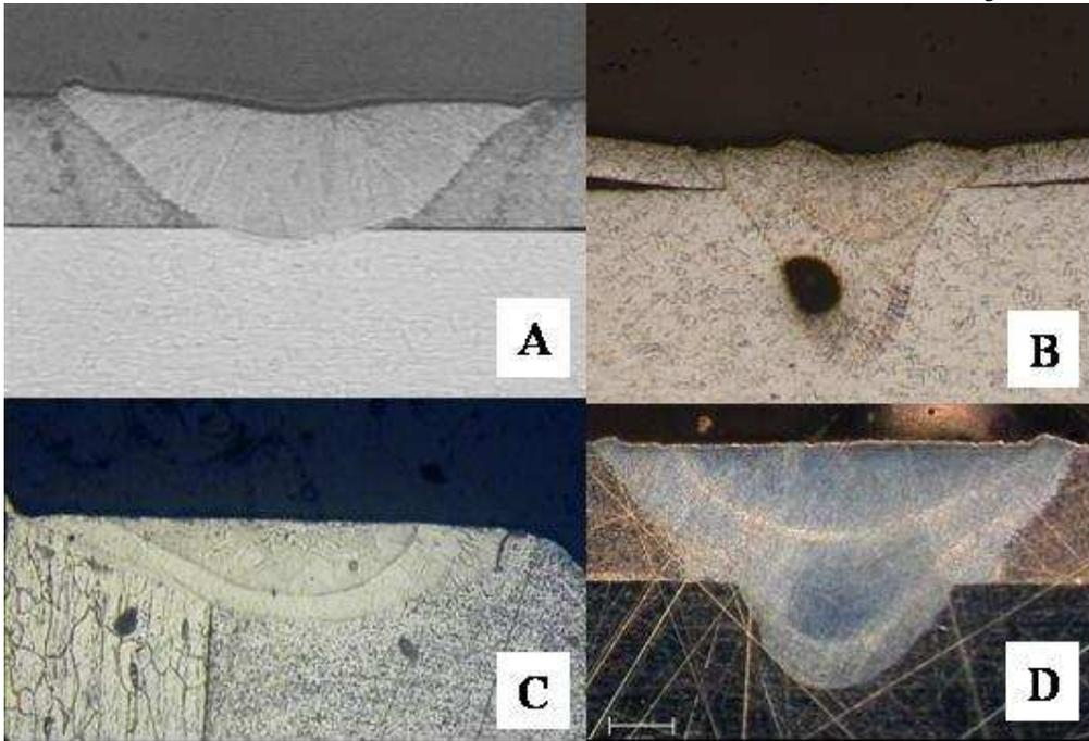
Figure 5. Laser weld cross-sections showing shallow conduction weld (A), pulsed keyhole weld (B), and weld sections affected by difference in thermal diffusivity (C) and reflectivity (D) of the two parts being welded.
