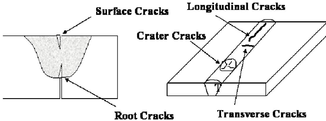
Figure 7. Schematic showing typical locations for crack formation during rapid cooling induced stresses. Other factors such as part restraint and materials could also affect residual stress and cracking.
