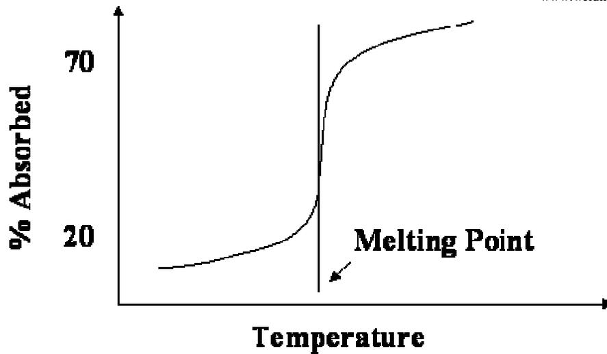
Figure 3. Schematic shows increase in laser absorption with temperature; absorption increases dramatically as the metal melts. The shape of the absorption curve varies for different metals but overall shape is similar.
