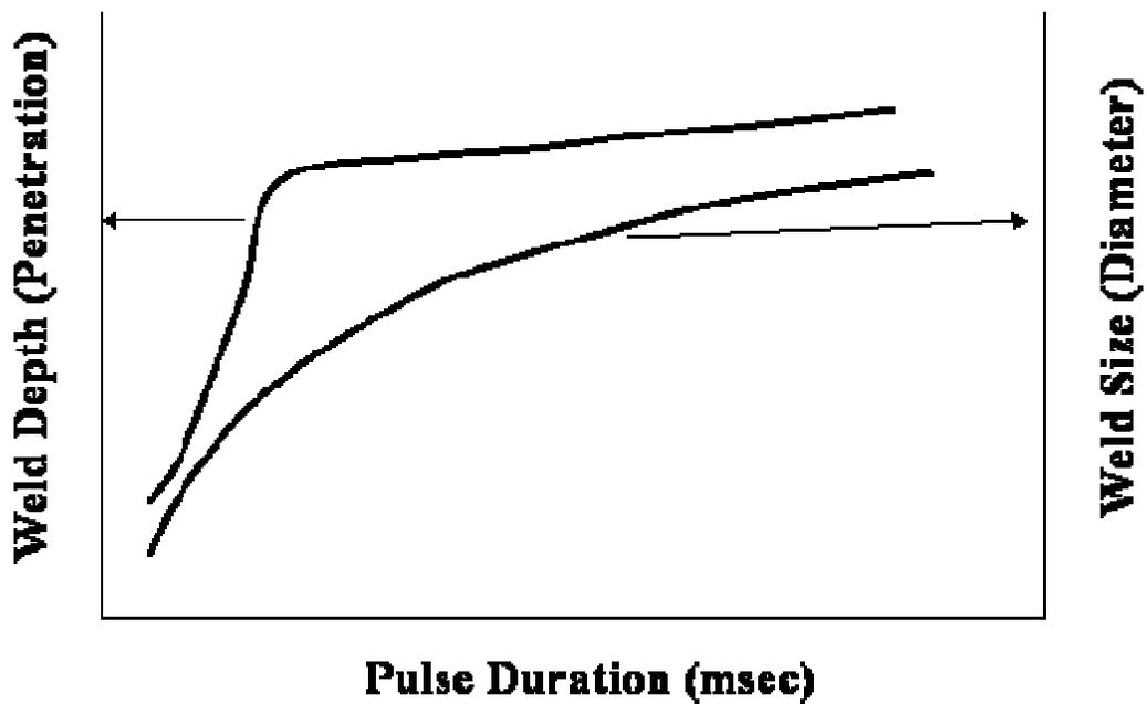
Figure 6. Graph showing effect of time on weld penetration and weld size at a given peak power.
