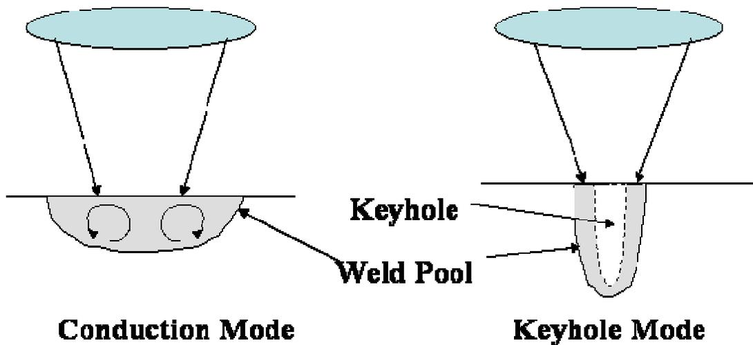
Figure 4. Schematic sections of welds in conduction and keyhole modes. Conduction mode welds are wide and shallow whereas keyhole mode welds are narrow and deep.
