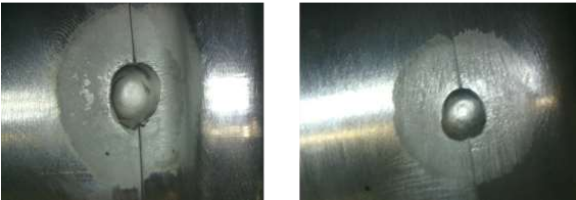
Figure 3. Shows two images of tack welds made on Aluminum with an AC balance of 60% (left) and 95% (right). The photo on the right with 95% AC balance has a minimal (5%) DCEP component and produces a much weaker frost effect which can be easily wire brushed to expose an almost pristine surface. In comparison, a 60% AC balance produces substantial frost which, on wire brushing, reveals significant surface melting.
