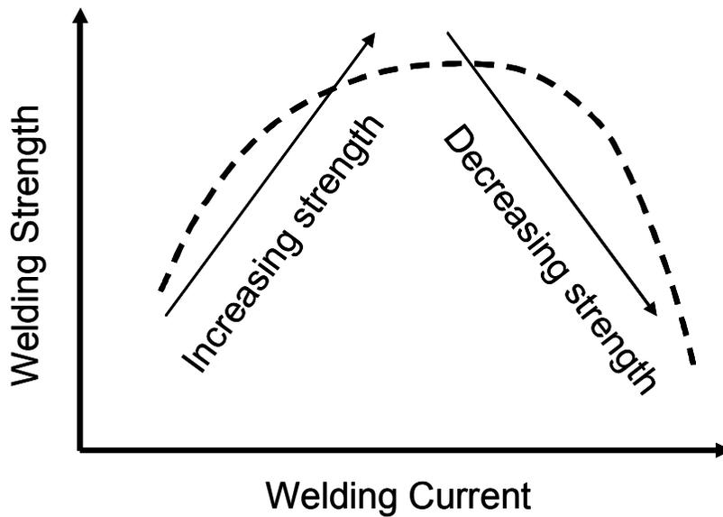
Figure 1. Figure shows a schematic of variation on weld strength as a function of welding current. To the left of the maxima, the welding strength increases with current; towards the right, it decreases with current.
