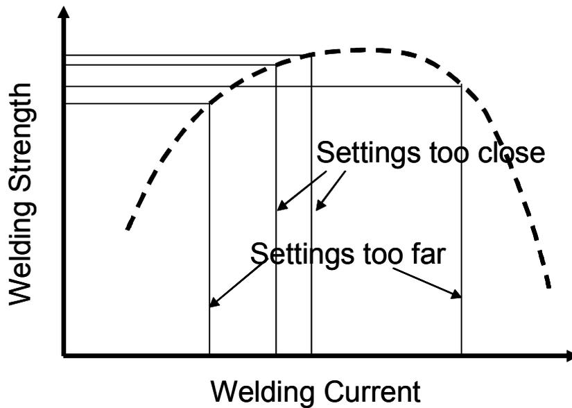
Figure 2. Figure shows a schematic with effects of factor settings. If factor settings are set either too close or too far, their effect on the output may not be significant and without process knowledge could lead to misleading results.
