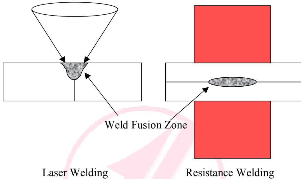
**Figure 1.** Schematic shows difference in heat generation between laser and resistance welding. The laser weld metal pool grows from the outer surface where as in resistance welding, the molten metal pool grows from inside out.
