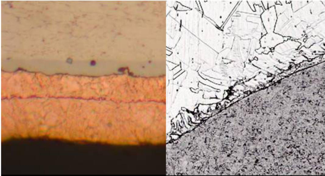
**Figure 3.** Photomicrographs of sections of solid-state bonds produced by resistance welding. Note the intact weld interface even after welding with no sign of fusion at the weld interface.
