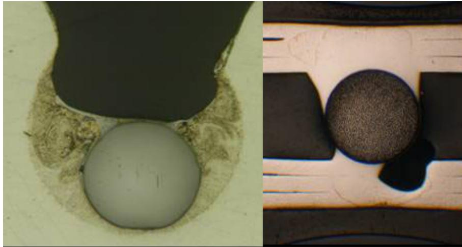
**Figure 2.** Photomicrographs of sections of joints formed by laser (left) and resistance welding (right) where one of the alloy is has much lower melting point and results in effectively forming a braze on the higher melting component.
