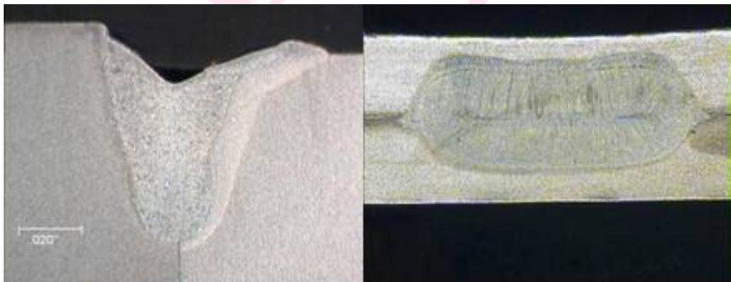
**Figure 4.** Photomicrographs of sections of fusion bonds produced by laser (left) and resistance welding (right).
